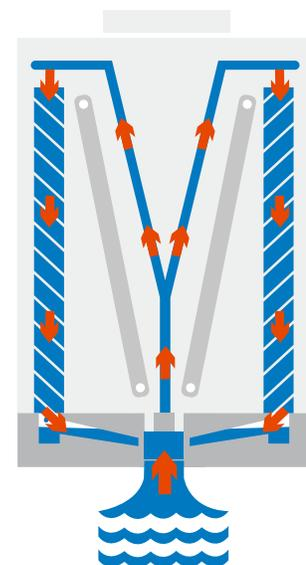
Water enters the unit and is circulated throughout, never remaining still. Every 2 hours, the water is drained from the unit, requiring no water treatment.
