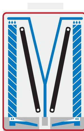
Once daily, fans reverse cooling direction and blow dirt and debris off the coil and Pre-Cooler Pads, sweeping the unit. Water then rises the pads, piping and basin and is flushed from the unit to maintain peak performance.
