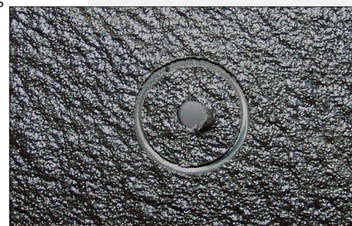
Figure 12. Scored TriArmor® Corrosion Protection System
