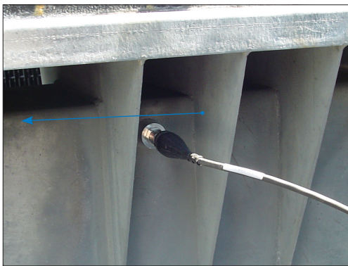
Figure 11a. Accelerometer Location - Gear Drive
