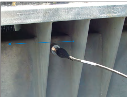
Figure 14a. Accelerometer Location - Gear Drive
