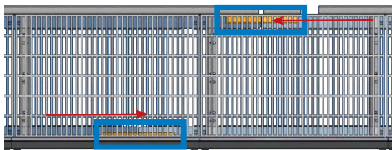
Figure 14. Move splice plates into positions shown
