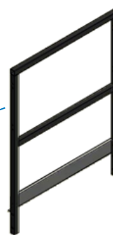
Figure 18. Field-installed A-Frame handrail section
