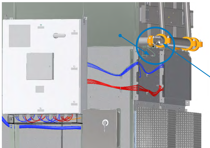
Figure 22. Manifold Connection Outlet and Leaving Process Fluid Temperature Sensor
