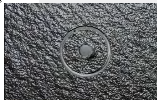
Figure 15. Scored TriArmor® Corrosion Protection System
