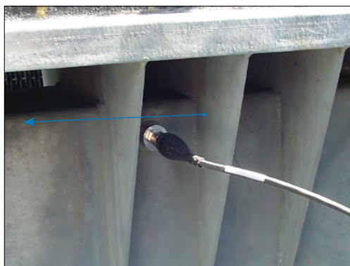
Figure 14a. Accelerometer Location - Gear Drive
