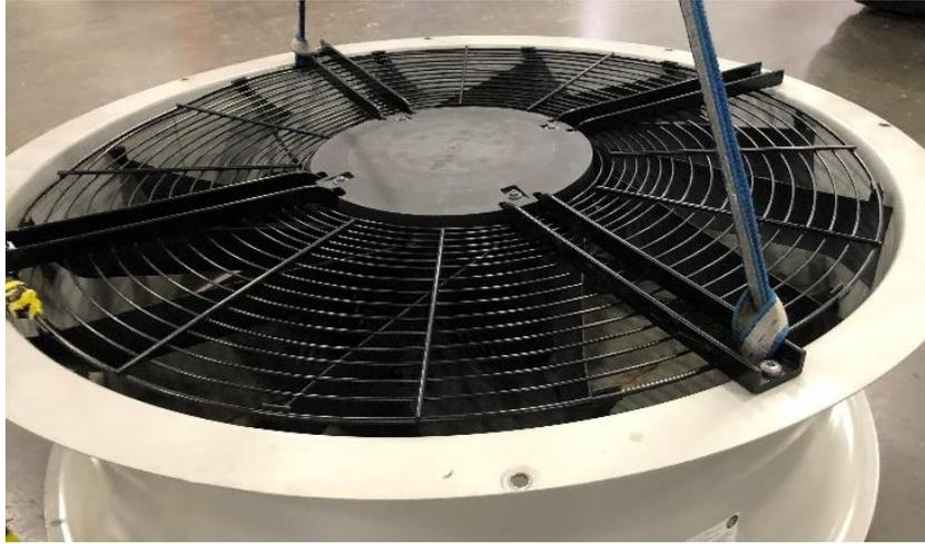
*Figure 19. Fan and Motor Assembly Lift*
