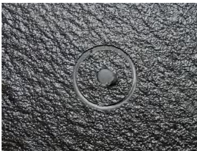
Figure 23. Scored TriArmor® Corrosion Protection System
