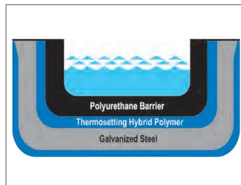
TriArmor® Corrosion Protection System Triple Layer Protection
