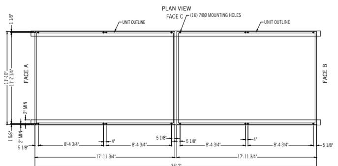
Plan A: S15E/XES15E-1218 Double Cell Unit
