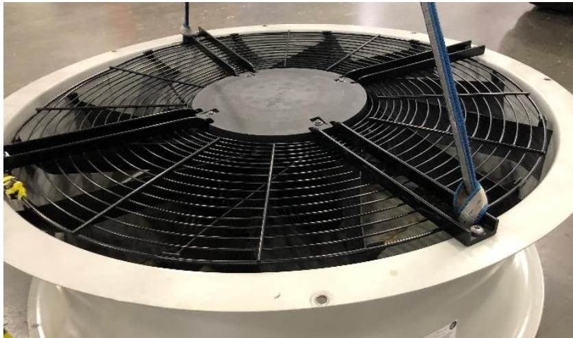
Figure 19. Fan and Motor Assembly Lift
