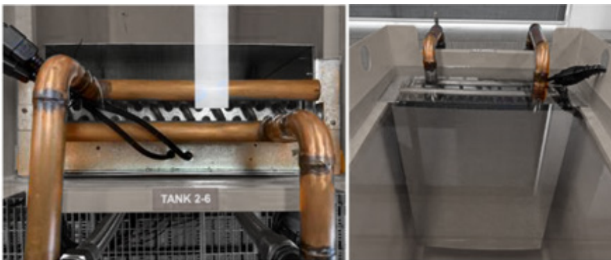
Figure 18: FCM properly supported over tank's internal railing
