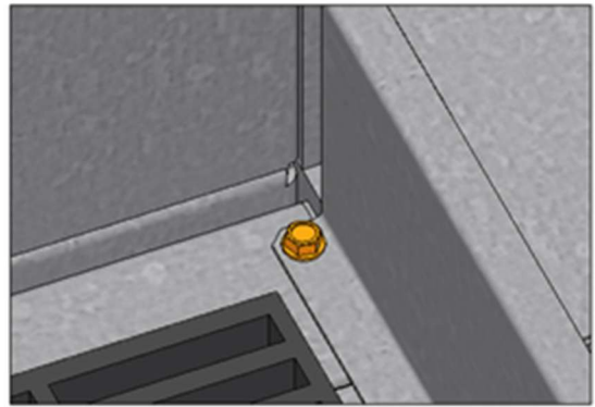
TOEBOARD TO PLATFORM 5/16 TAPPER (1 PLACE)
