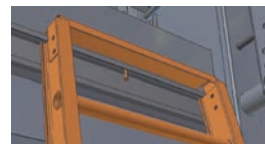
Detail B. Upper Ladder Support
