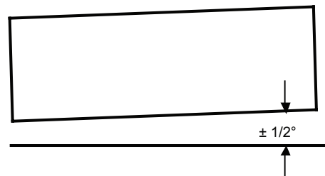
Figure 16. Coil Module Level Tolerance as Seen from the Plenum Side
