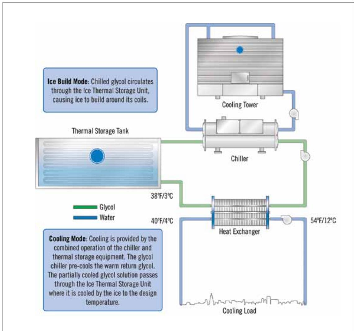
>> Details of how an ice thermal storage system operates.
