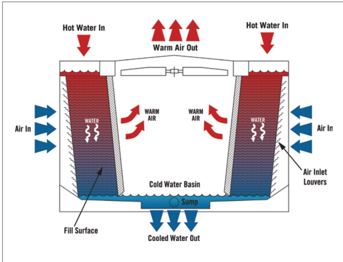
nance and smooth, reliable year-round operation. A cross-flow cooling tower typically meets these objectives and can provide an excellent method of campus cooling.
