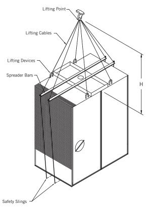
Figure 2. Rigging of All FXT Models Except for FXT-58 and FXT-68
