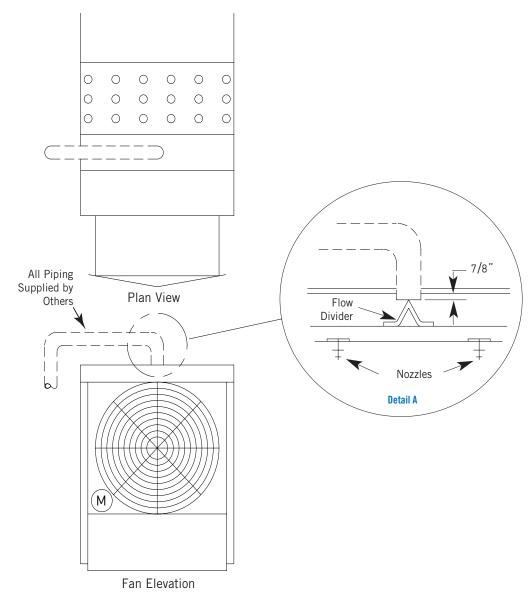
Figure 3. Top Inlet Piping Installation
