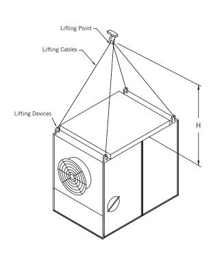
Figure 1. Rigging of Models FXT-58 and FXT-68
