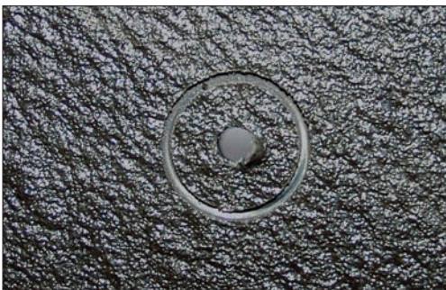
Figure 11. Scored TriArmor® Corrosion Protection System
