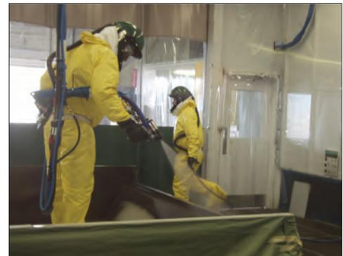
Application of TriArmor® Corrosion Protection System
