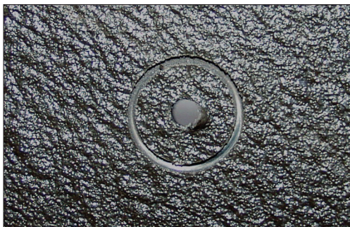
Figure 12. Scored TriArmor® Corrosion Protection System
