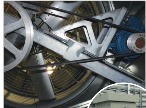
BALTIDRIVE® Power Train Used for VFD Applications
