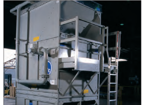
External Platform and Ladder
