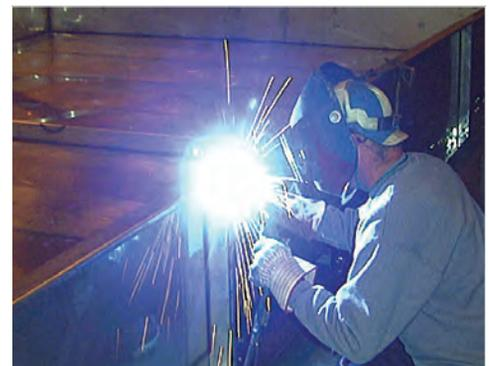
Welded Stainless Steel Cold Water Basin
