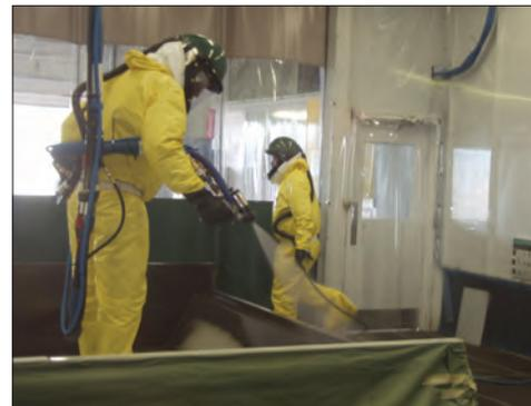
Application of TriArmor® Corrosion Protection System
