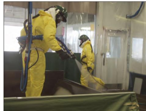
Application of TriArmor® Corrosion Protection System
