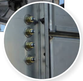
Extended Lubrication Lines with Grease Fittings Located by the Access Door
