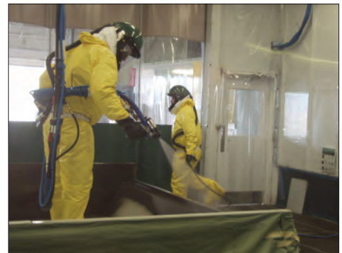
TriArmor® Corrosion Protection System Spray Booth
