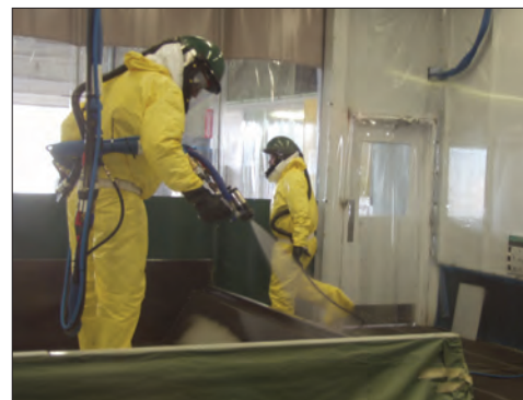
Application of TriArmor® Corrosion Protection System
