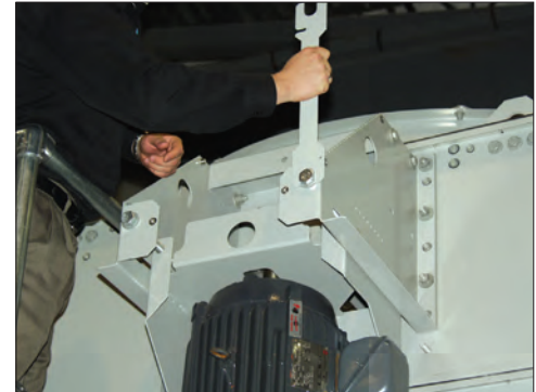
Standard BALTIDRIVE® Power Train Externally Mounted Motor Models PT2-0709A, PT2-0809A, and PT2-0812A
