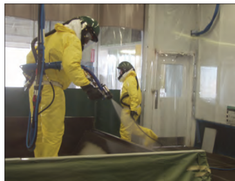
Application of TriArmor® Corrosion Protection System
