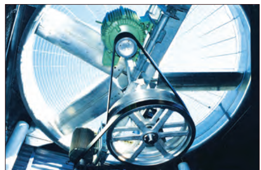
Mechanical Belt Drive System
