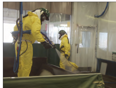
Application of TriArmor® Corrosion Protection System
