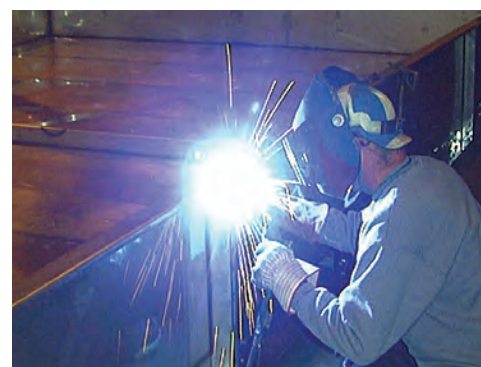
Welded Stainless Steel Cold Water Basin
