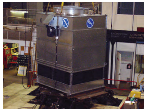
PT2 During Shake Table Testing
