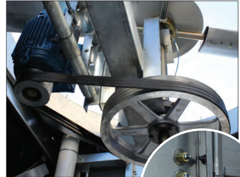
Extended Lubrication Lines with Grease Fittings Located by the Access Door
