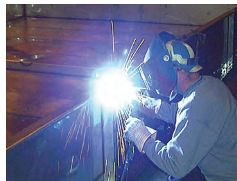
Welded Stainless Steel Basin
