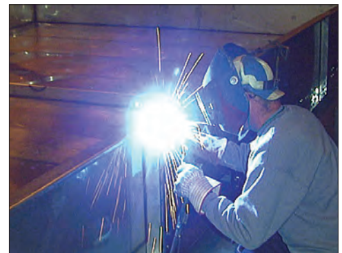
Welded Stainless Steel Cold Water Basin
