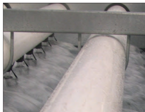
Non-clog Nozzles Ensure Even Flow Over Coil Area
