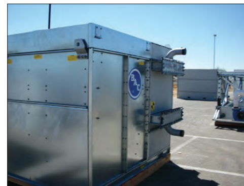
Cleanable Header Coil
