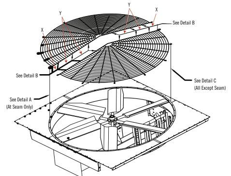
Figure 13. Two-Piece Fan Guard Assembly
