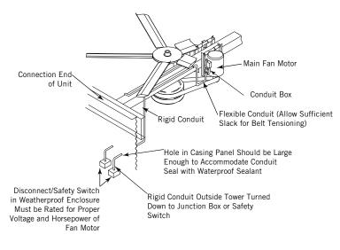
Figure 18. Belt Drive Motor Location(s)
