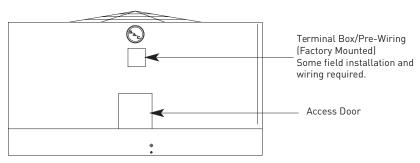
Figure 23. Factory Pre-Wired Terminal Box Location
