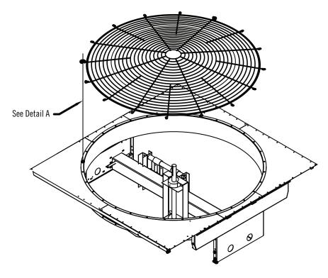
Figure 12. One-Piece Fan Guard Assembly
