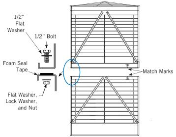
Figure 3. Upper and Lower Assembly for Series 5000 Cooling Towers
