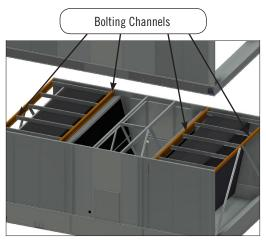
Figure 6. Bolting Channels
