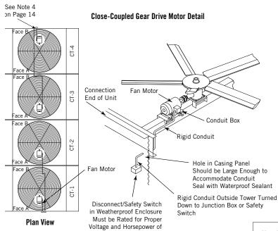
Figure 19. Motor Location For Close-Coupled Gear Drive
