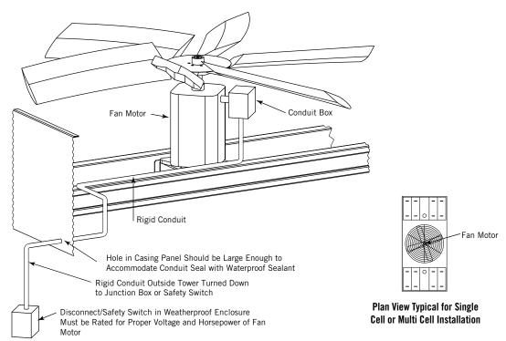
Figure 21. Motor Location For the ENDURADRIVE® Fan System
