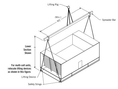
**Figure 2.** Lifting Instruction for Multi Cell Units: One Section Cells or Two Section Cells (Lower Section Shown)
