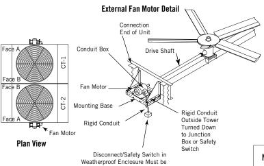
External motor, mounting base and drive shaft must be field-installed. Drive shaft must also be properly aligned after installation by qualified personnel to ensure satisfactory operation.
