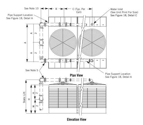
Figure 15. Single Riser Piping Schematic
