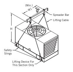
**Figure 1.** Lifting Instruction for Single-Cell Units: One Section Cells or Two Section Cells (Upper Section Shown)
