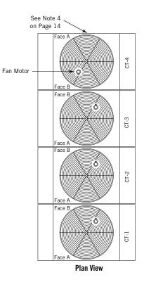
Motor Detail for Main Motor (BALTIDRIVE® Power Train)
