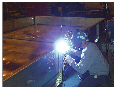
Welded Stainless Steel Basin
