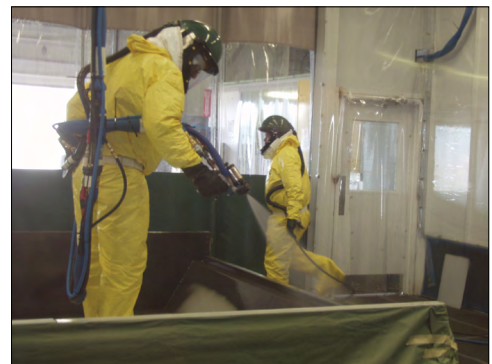
Factory Application of TriArmor® Corrosion Protection System
