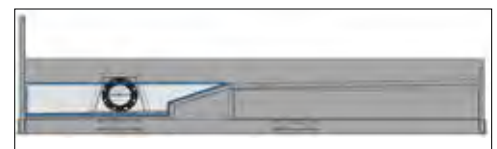
Vertex Evaporative Condenser Basin 30% Lower Water
