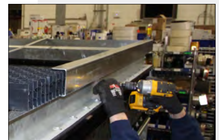
Figure 10. CIS Hail Guards - Loosen and Remove Hardware from End Covers
