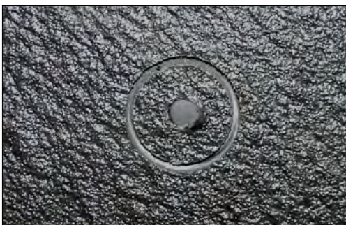
Figure 12. Scored TriArmor® Corrosion Protection System
