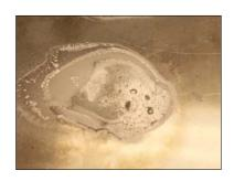
Chemical Corrosion Test Shows Durability of Type 304 SST
