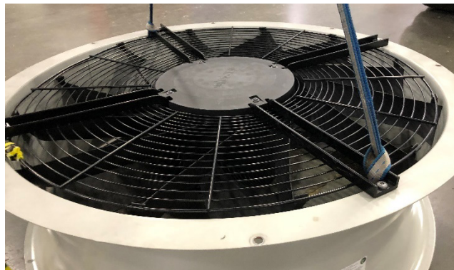
Figure 24. Fan and Motor Assembly Lift
