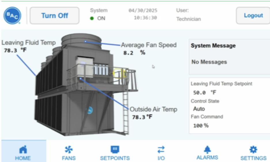
4. All four (4) fans in the unit will turn on, ramping up to 100% speed. Each fan may not start at exactly the same time as the others. It may take a fan approximately 45 seconds to ramp up from
