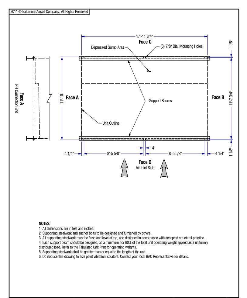
CXVB Evaporative Condenser Plan "A" Steel Support Print
